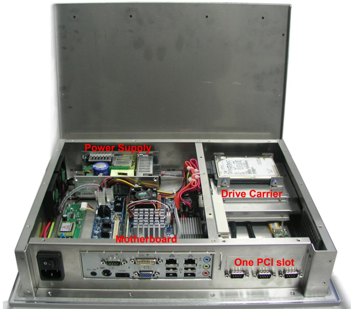
Internal Component Locations (Fomax F1 Series – 1 PCI Slot Model)
