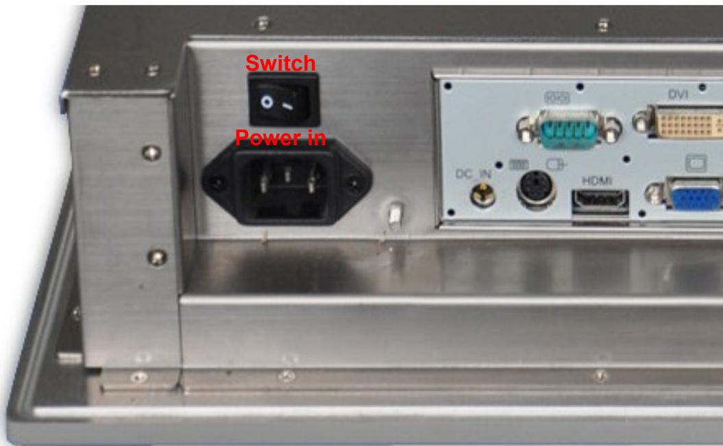
The Nematron Fomax industrial Fanless PC uses an 12VDC Power Supply. The input socket is located on the left side panel of the chassis. We would supply an adapter with auto-ranging 100-240VAC, you can uses the adapter or 12VDC power input directly.
